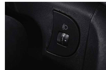
Angle controllable Headlight switch.
