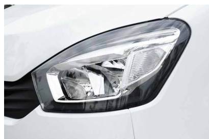
Headlight cluster with integrated LED Daylight for enhanced aesthetics and safety operation.
