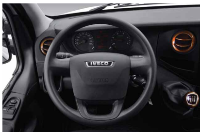
Nodding steering wheel with 4-way adjustment.
