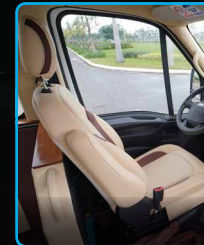
Driver seat 6-way adjustment, ensuring driver visibility and comfortable.
